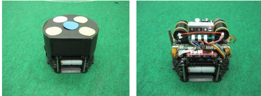
Fig. 1. RoboDragons new robot (Left: with cover, Right: without cover)
