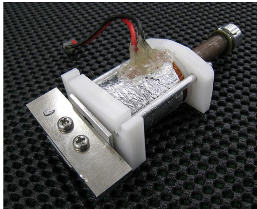
Fig. 2. Column type kick device
