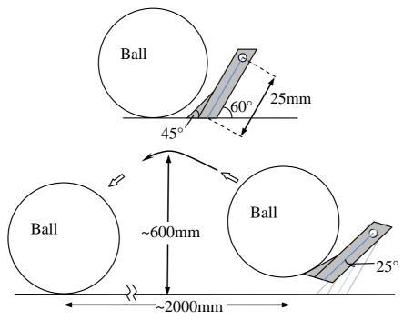
Fig. 21 Specification and performance of actual chip-kick device
