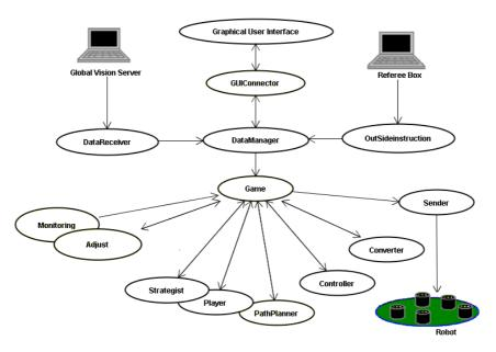
Fig. 10 Schematic diagram of strategy system
