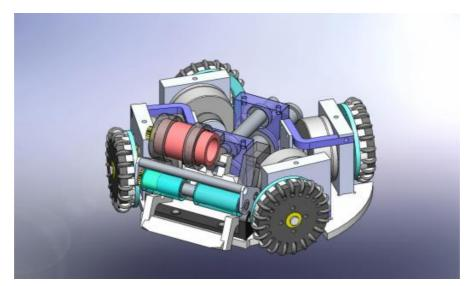
Fig. 15 Whole mechanical design
