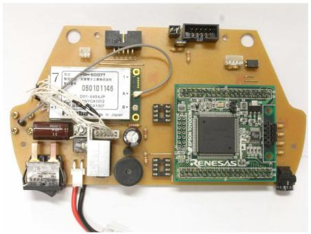
Fig. 3 Main electronic board
