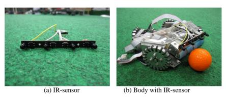
Fig. 23 Detecting device (IR-sensor) for a ball
