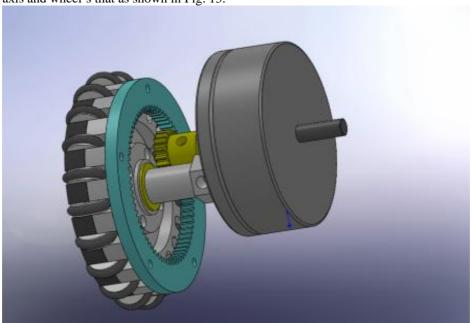
Fig. 13 Ring-wheel and internal gear
