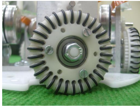
Fig. 2. Locomotion system: omniwheels.
