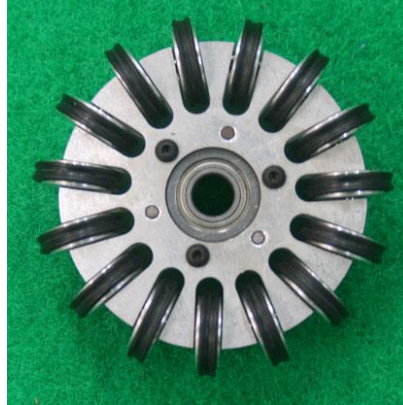
Fig. [12]. Real omni-directional wheel used in Skuba 2009 robot.
