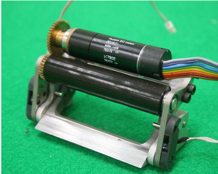
Fig. [15]. The dribbling system.
