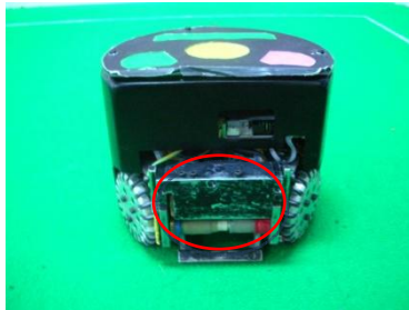
Fig.5 The front view of the robot and overview of the dribbler
