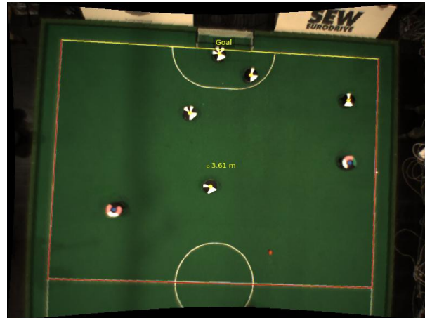
Fig. 7. Distortion corrected camera image with field lines
