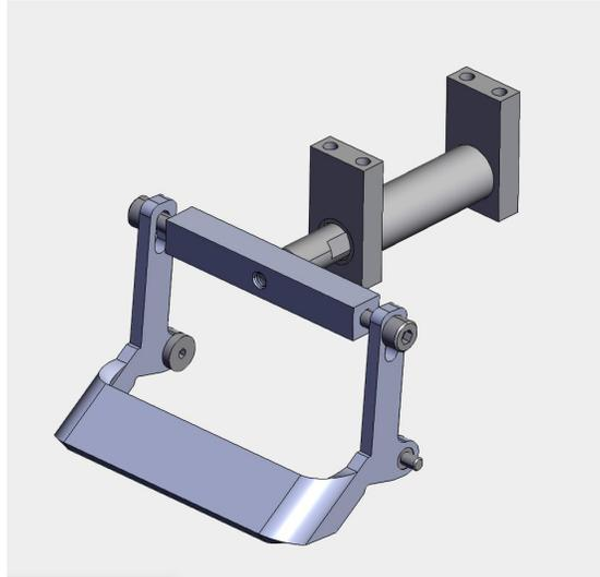
Fig. 2.2: Simplified CAD Model of New Chipper/Kicker Design
