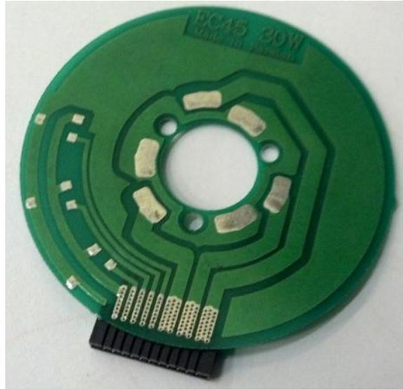
**Fig. 6.** Parsian made motor PCB
