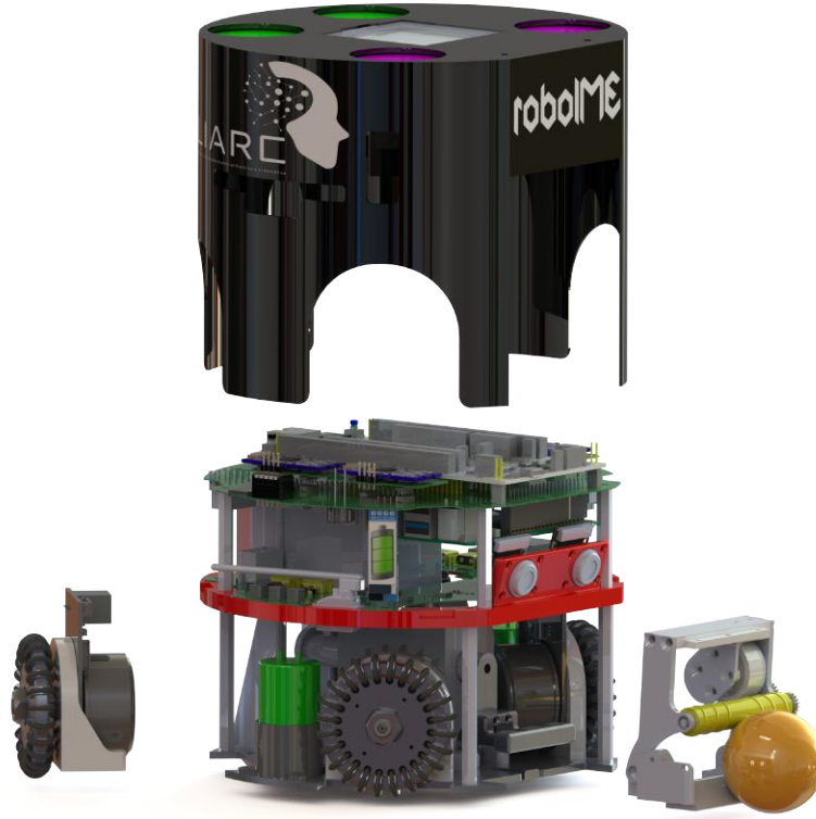
Fig. 1: Full robot exploded view
