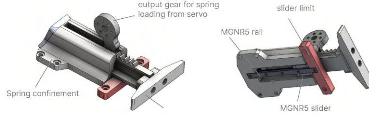
Fig. 11. Spring loaded linear kicker assembly
