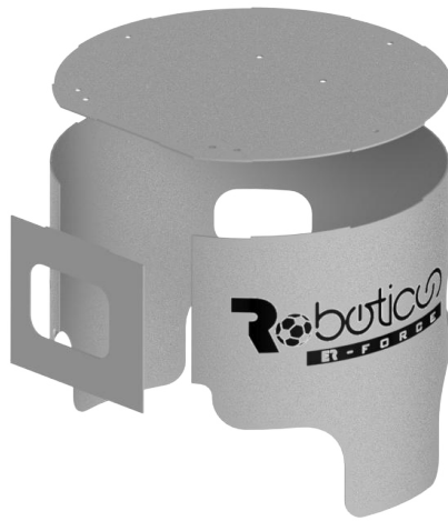
Fig. 3: Exploded view of the cover
