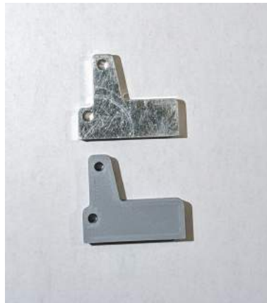
Fig. 1. Comparison of original super stands with 3D printed prototype.
