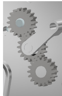
Fig. 6. Triple gear system for the dribbler.
