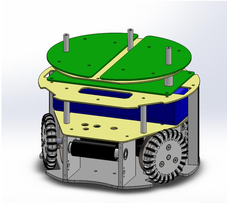
**Fig. 1.** Internal mechanical assembly of the 2019 Warthog Robotics SSL robot (same of last years).
