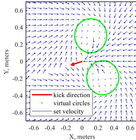
**Fig. 4.** Set velocity in the output ball interception algorithm at different robot locations
