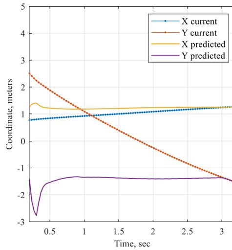
**Fig. 3.** Prediction of ball coordinates with initial prediction interval set to 3 seconds.
