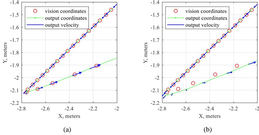
Fig. 1. Raw vision data and the output of Kalman filter (a) after and (b) before the update.
