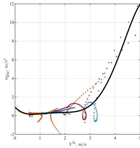
**Fig. 2.** Estimated rolling friction deceleration as a function of ball speed (solid curve) and interpolated data acquired from several recorded free-roll fragments (dotted curves).
