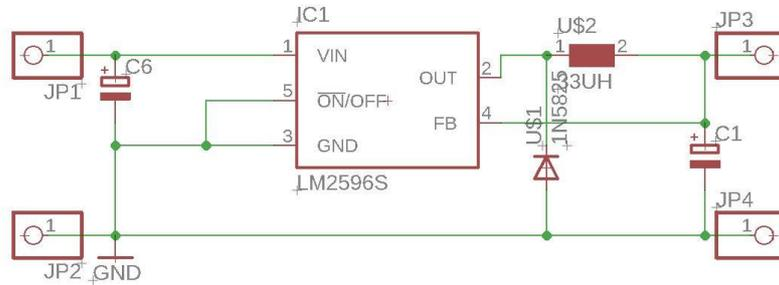
**Fig. 6.** LM2596 Circuit Schematic.
