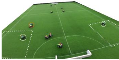
Fig. 2. Attacker shown in the red circle has the ball with the other two teammates located in their assigned dynamic zones.
