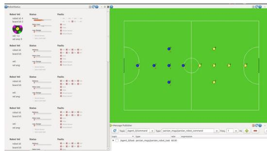
**Fig. 10.** Robot status and monitor widget in rqt
