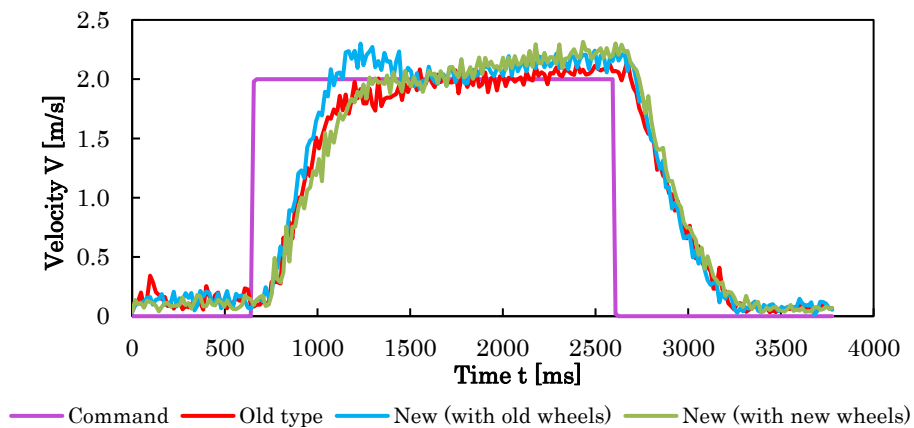
Fig. 9. Robot speed from a stop to 2 meters per second
