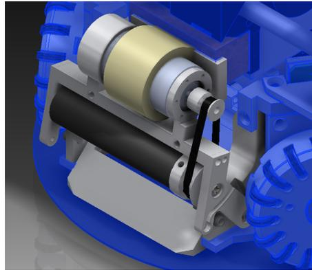
**Fig. 4.** The new Dribbler Mechanism
