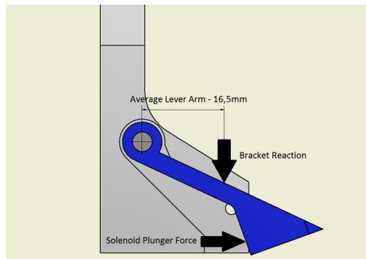
**Fig. 7.** New Chip Kick Diagram
