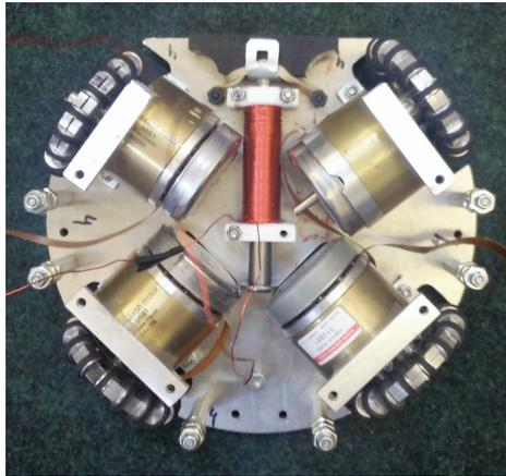
Fig. 5: Motors and kicker attached to chassis
