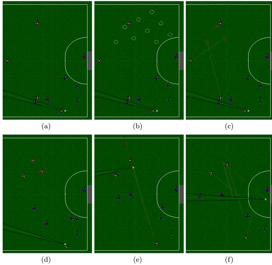
**Fig. 7.** a) Initial setup for servicing a free kick for the STOX's team. b) Locations found by the described algorithm are shown in white circles on the field. c) Three selected locations shown in red circles to send the three available attackers. d) The three attackers has been placed in to the three selected locations. e) The pass is made to the attacker with higher scoring chance. f) The attacker receives the pass and shoots at goal, finally scoring.
