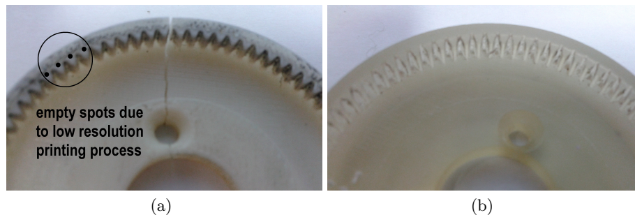
Fig. 3. (a) Cracked gear (lower precision). (b) Stereolithography printed gear.
