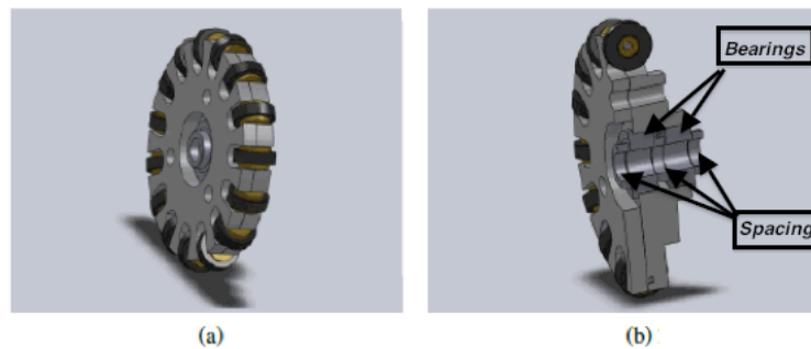
Fig. 4: 2011 Drivetrain Wheels: (a) Custom Wheels (b) Assembly Details
