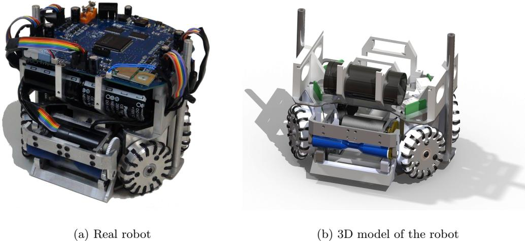
**Fig. 1.** Real robot picture and its mechanical 3D model view
