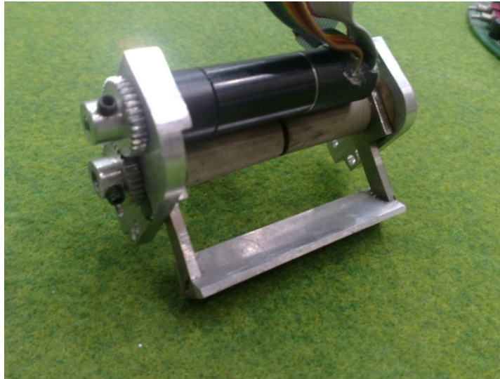
Fig. 8. The spin back and chip kick system.
