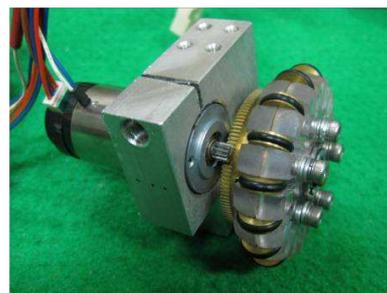
Figure 2. Motor, gear, and wheel assembly.
