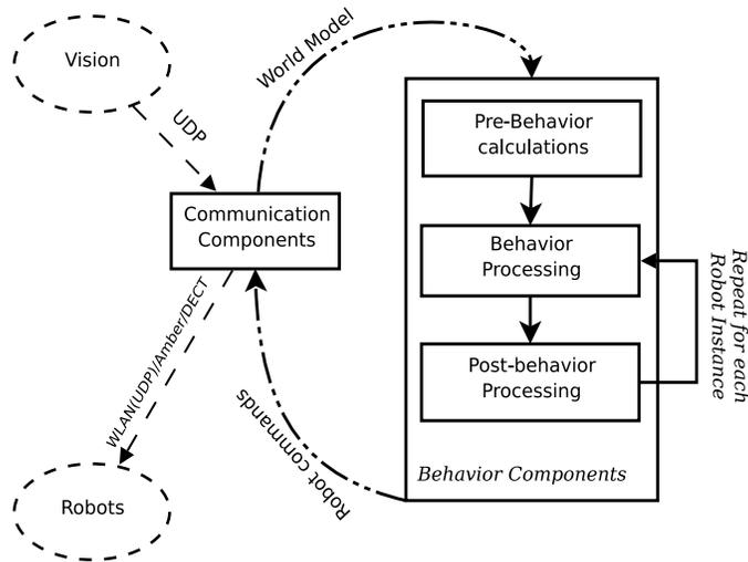
**Fig. 3.** Main loop structure of the agent software
