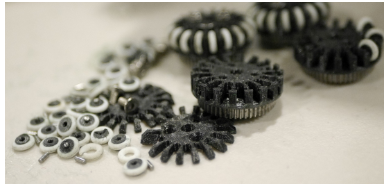
Fig. 3: v2019 robot wheels after RoboCup 2019 in Sydney. Most wheel covers are broken and could not retain their subwheels.
