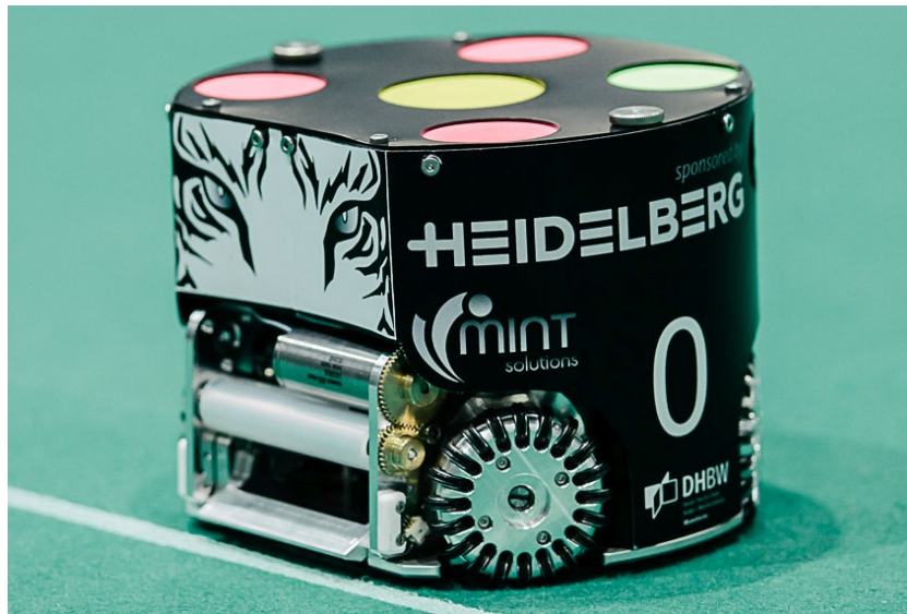
Fig. 1. New robot with cover on the field (v2016). Sub-wheels are completely covered by each wheels top plate to prevent direct impacts.
