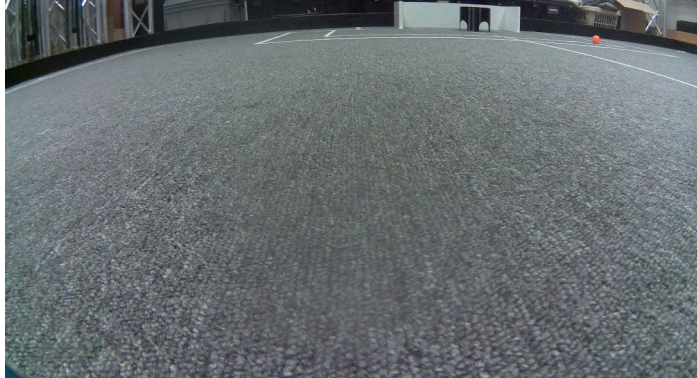
Figure 5.7: The carpet at close proximity shows the inconsistent shading caused by uneven dye and the carpet pattern. This leads to random blobs of similar shading with varied sizes up to robot pattern and ball sized blobs.
