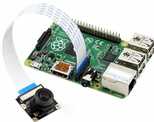
**Figure 2.2.:** Raspberry Pi 3 and the Raspberry Pi Camera Module [12]
