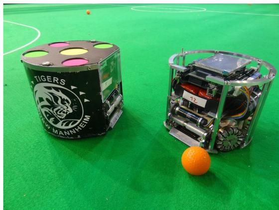
Figure 1: Two robots from Tigers Mannheim. The left robot has a colored pattern attached that is used to track the robots position, orientation and id.
